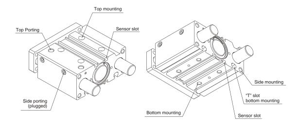
These guided compact cylinders, characterised by reduced overall dimensions, can be used for the compression, conveyance and manipulation of objects in many industrial sectors; similarly they can also be used in pushing, lifting and stopping applications.
