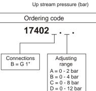
Example: **17402B.C** Pressure regulator with G 1" connections, adjusting range 0 - 8 bar with relieving.
