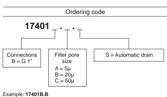
Filter size 3 with G 1" connections and filter pore size 20µ.
