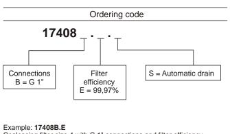
Coalescing filter size 4 with G 1" connections and filter efficiency of 99,97%.
